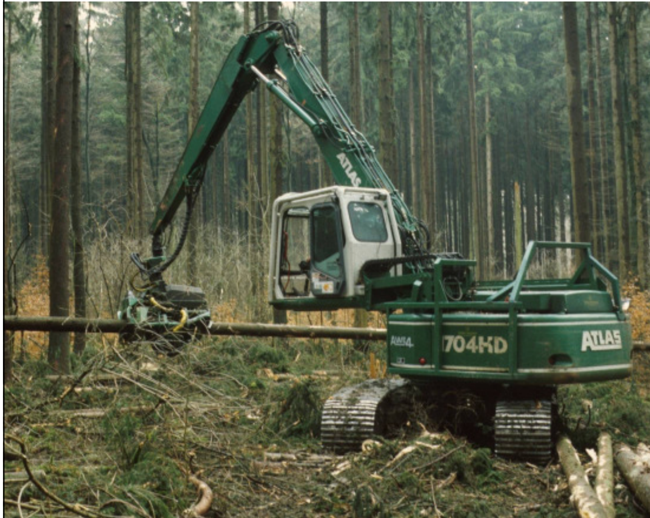
Large-sized track harvester (excavator chassis)
